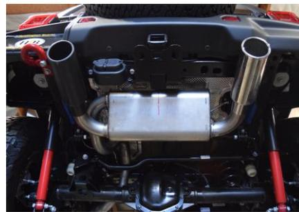
Slide the 2.5" band clamp over the expanded part of the muffler and make clamp snug but not tight. Install the Gibson provided tips. Check for exhaust clearance before tightening.
