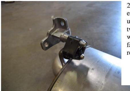
2. Remove the factory exhaust hangers from the using a 13 mm removing the two bolts. These hangers will remain attached to factory muffler when being removed
