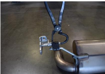
Remove hangers from OEM exhaust using removal pliers or large channel pliers and re-install them on the Gibson as shown. Using a lubricant can aid in the removal.
