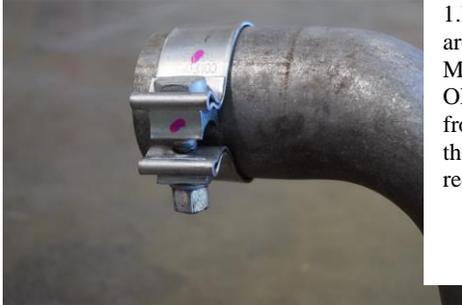
1. Be sure to check all parts are correct and match the Manual. Loosen the factory OEM clamp located just in front of the muffler above the factory axle. This will require a 15MM.
