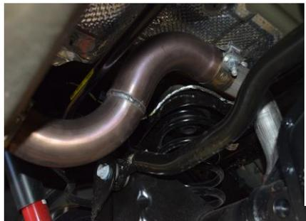
3. Once you have removed the OEM exhaust install Item# E onto the factory oem pipe. Use clamp # b to secure. Be sure notch is lined up and do not tighten clamp.
